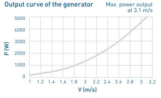
Power curve tested at towing tank of SVA Potsdam. Results may vary in natural rivers & canals. Curve was measured at the generator output.
